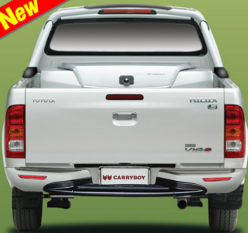
CB-734 Rear Nudge Guard RTM Produced from a premium grade material by RTM system with anti-slip rubber pad and the rear red reflector.
