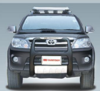
**CB-705 PU. Front Nudge Guard** Produced from high quality polyurethane with center aluminum
