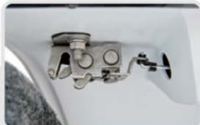
Locking System Double action rotary lock.
